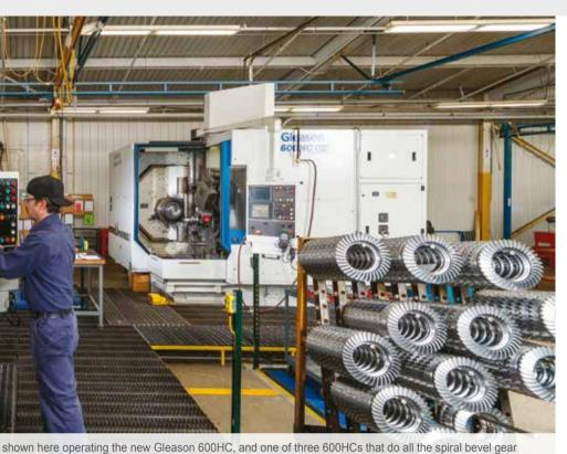
re operating the new Gleason 600mG, and one of three 600mGs that do all the spiral bever gear
