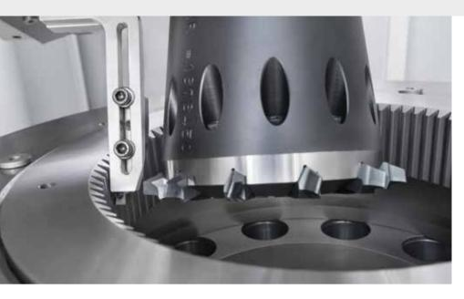
The Hard Power Skiving machines are equipped with a stock dividing sensor to detect the position of the tooth gap.
