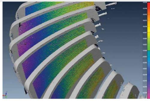
3D laser scan of bevel gear showing traces of cutting marks which even if in tolerance can potentially result in negative noise characteristics.
