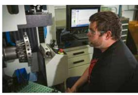
Once the operator has loaded the cutter head, positioned the build carriage and loaded the blades, he's free to perform other tasks while the 500CB completes the build, truing and inspection operations.
