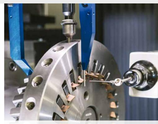
Gleason 500CB Cutter Build Machine eliminates costly tool room bottlenecks and frees up valuable manpower by automating time-consuming cutter build and inspection operations.
