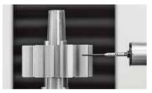
Surface roughness measurement, to help ensure consistently high-quality surface finishes.
