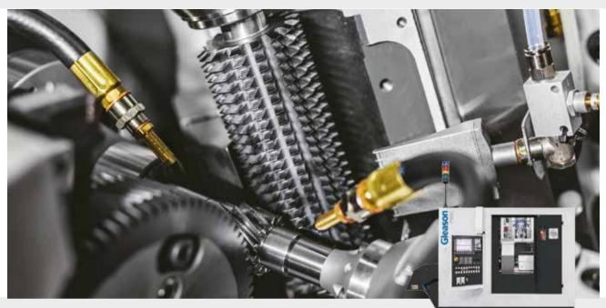
A two-cut process is executed in a single setup (cutting-chamfering/ deburring-cutting) and eliminates secondary burrs and residue on the gear flanks. It benefits subsequent hard-finishing processes and protects the tool life of expensive finishing and dressing tools, particularly honing.
