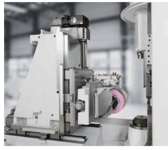
Double spindle concept for short idle times.
