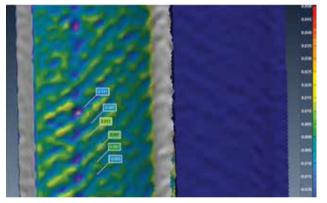
In this Power Skiving scallops analysis, depicting variations on the gear tooth aid in making corrections to reduce noise and tool wear.
