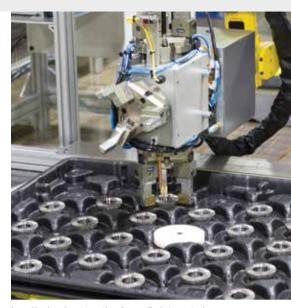
Load/unload automation is easily integrated with the 280G, further reducing nonproductive time.
