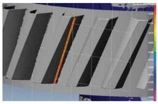
3D point cloud generated by non-contact laser probe in a single scan is analyzed and true deviations along line of contact are extracted...
