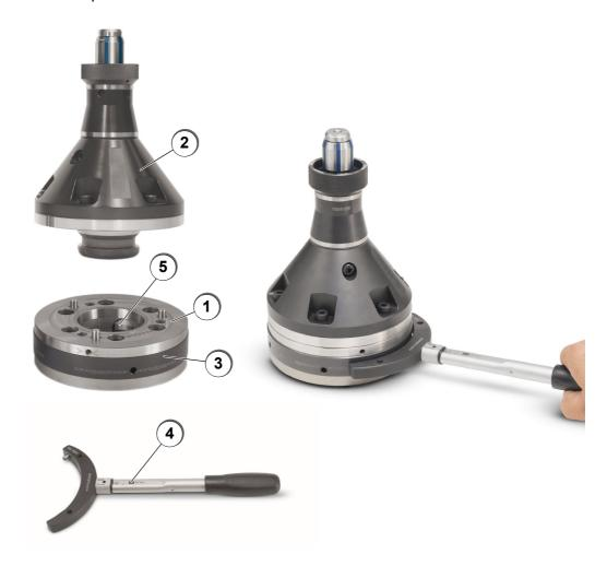
To change the clamping device (2) only the enclosed actuation wrench (4) is needed. With a turn (approx. 90°) of the actuation wrench (4) the clamping device (2) is engaged and locked on the Quik-Flex® Plus (1).
