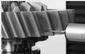
Tactile probing, for the complete inspection of a wide range of gear types, gear cutting tools and even non-gear, CMM-type measurement.
