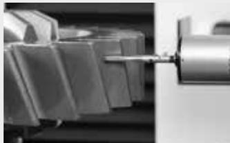
Surface roughness measurement, to help ensure consistently high-quality surface finishes.
