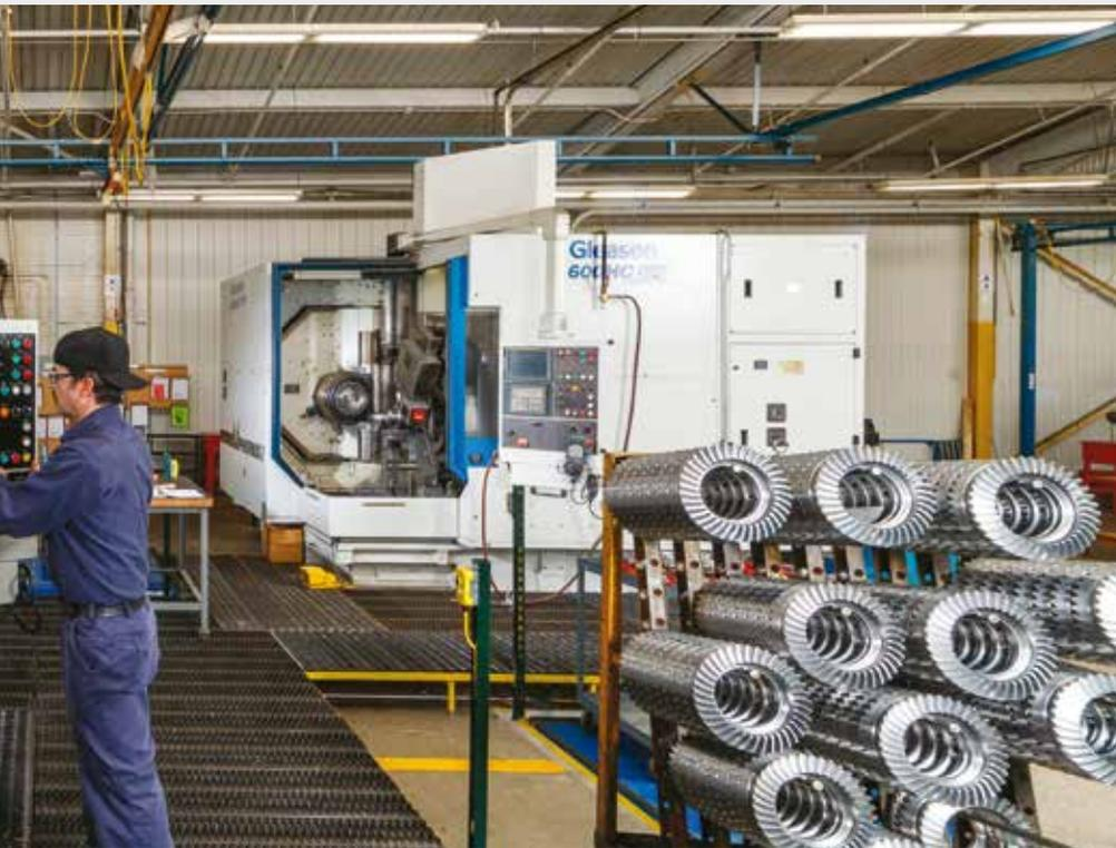
shown here operating the new Gleason 600HC, and one of three 600HCs that do all the spiral bevel gear
