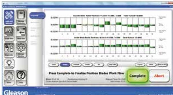
Blade position and runout are charted in real time, enabling the operator to easily monitor a build as it progresses.
