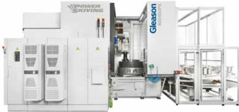
configuration, the 100PS is dedicated for shaft and internal gear applications.
