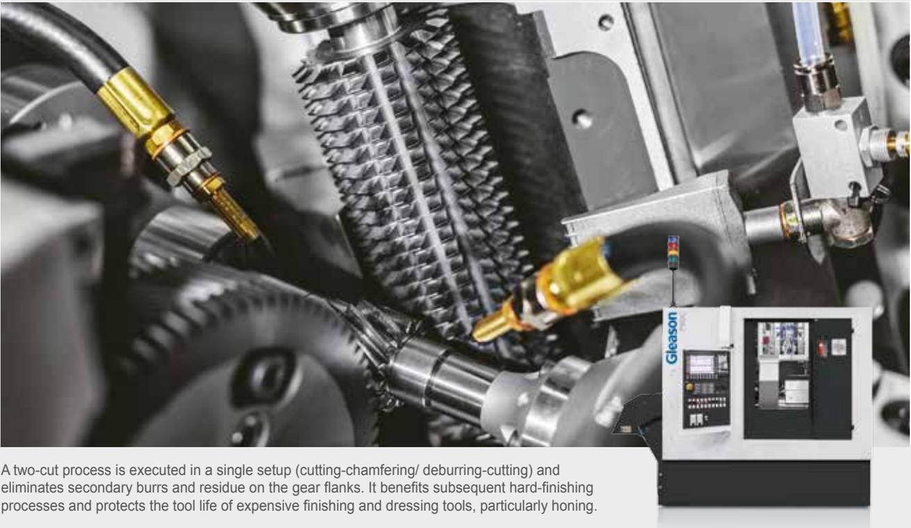
A two-cut process is executed in a single setup (cutting-chamfering/ deburring-cutting) and eliminates secondary burrs and residue on the gear flanks. It benefits subsequent hard-finishing processes and protects the tool life of expensive finishing and dressing tools, particularly honing.
