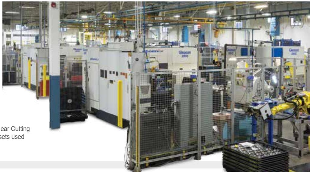
SEW Eurodrive relies on Phoenix® 280CX Bevel Gear Cutting Machines to produce most of the spiral bevel gearsets used in the popular K Series gear units.
