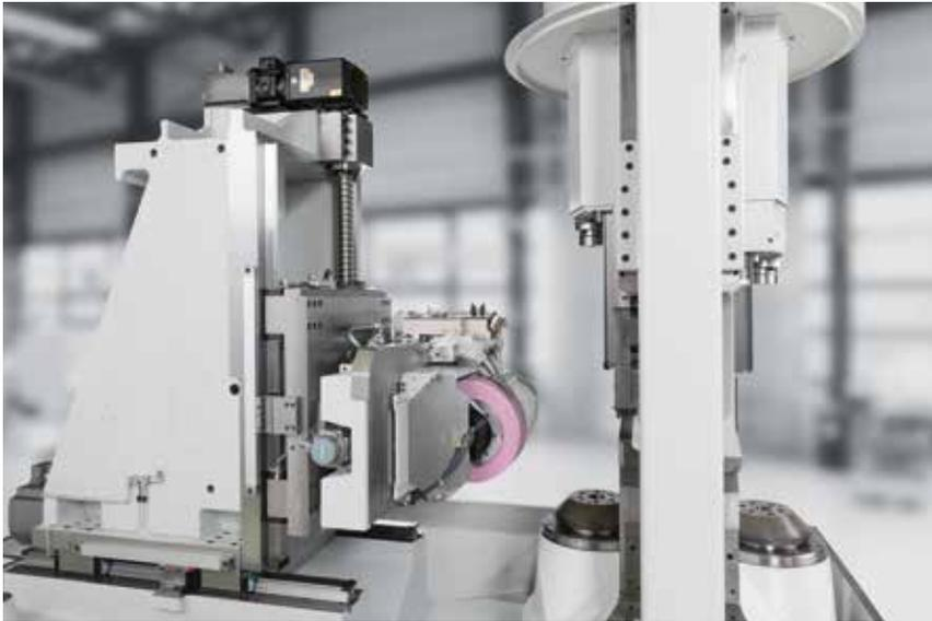
Double spindle concept for short idle times.
