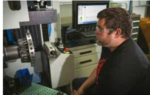
Once the operator has loaded the cutter head, positioned the build carriage and loaded the blades, he's free to perform other tasks while the 500CB completes the build, truing and inspection operations.
