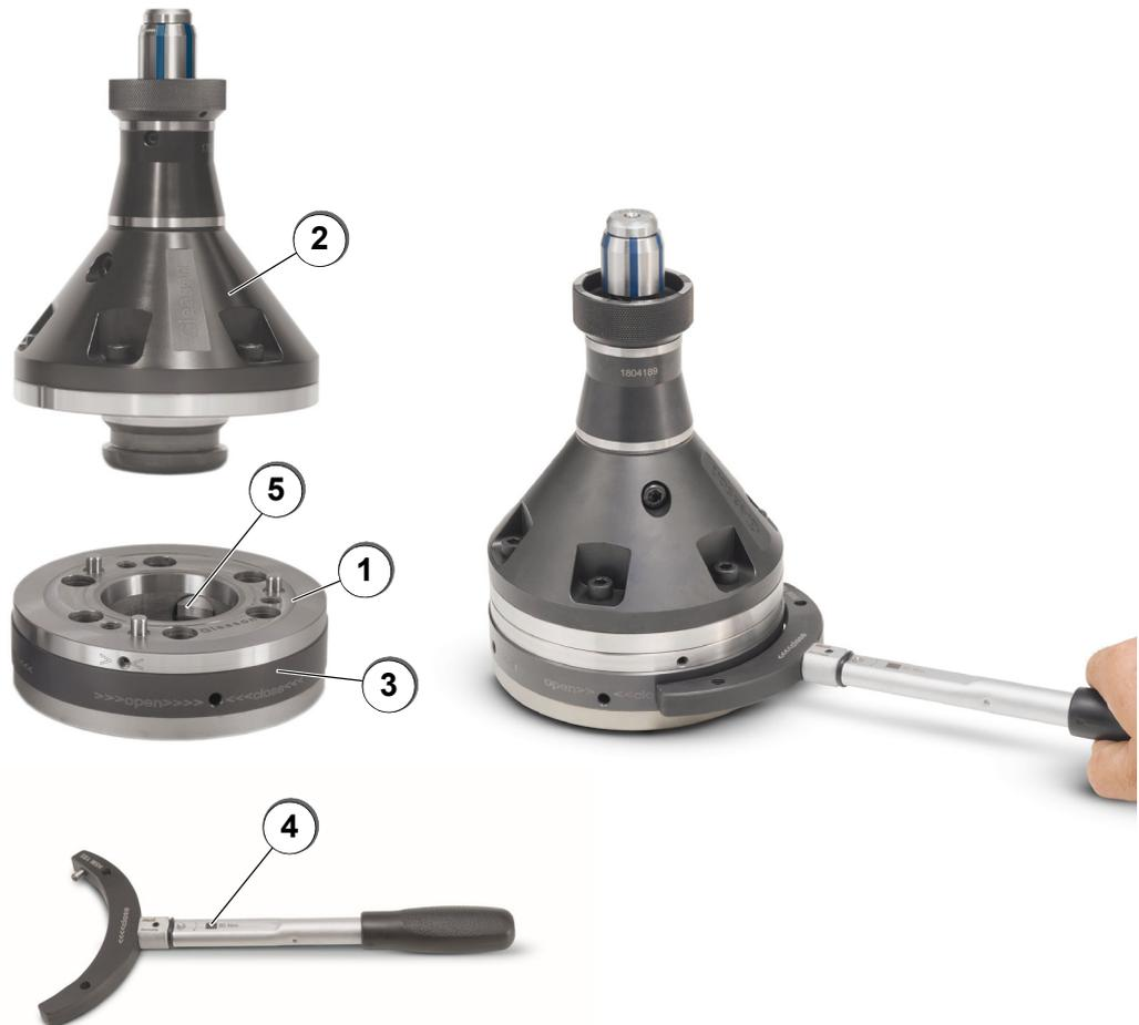
To change the clamping device (2) only the enclosed actuation wrench (4) is needed. With a turn (approx. 90°) of the actuation wrench (4) the clamping device (2) is engaged and locked on the Quik-Flex® Plus (1).
